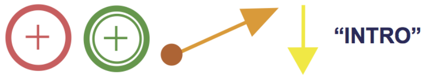
Figure 5.3: DemoWiz visualizes input events in a graphical way. From the left to right we show a mouse click, double-click, a drag, a mouse scroll, and keystroke events. These glyphs are overlaid on the video recordings.
